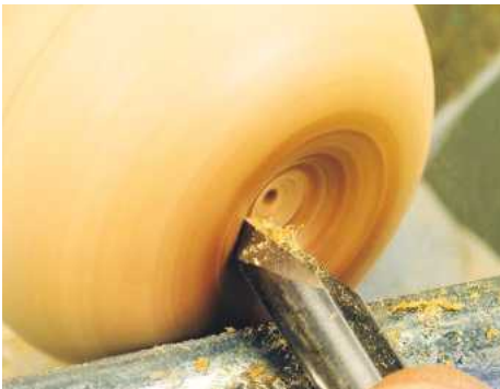
▲ Pic.9 He has swung the tool all the way around and into the end of the apple; don't push too hard in case you go across the centre of the work
